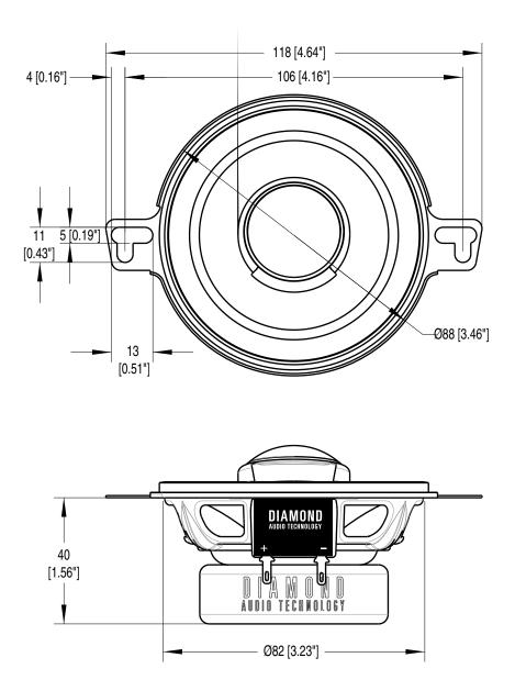
M341, M341i General dimensions in millimeters and [inches]. Not to scale.
